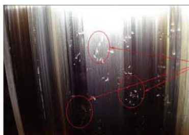
Wheel tread surface damages
